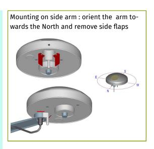
Option: Mounting bracket to fix Nano WSC11 box also on pole
