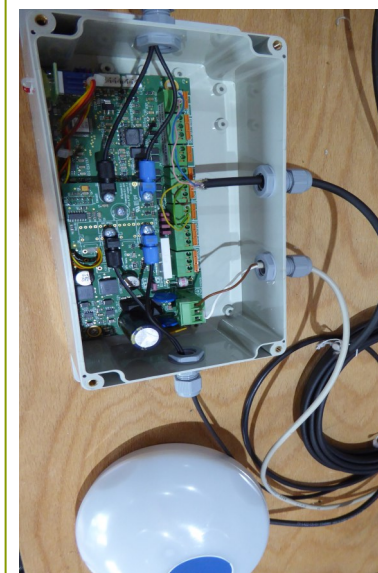
Picture of connecting nano with Thies WSC11
