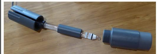
Install the holder in the pipe line. Take the pH sensor out of the transport tube. Insert it in adaptor tube with flat side on top in the holder. Slip the long screw top on the coax cable and screw it handtight without using force: glass!
