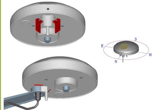
Option: Mounting bracket to fix Nano WSC11 box also on pole
