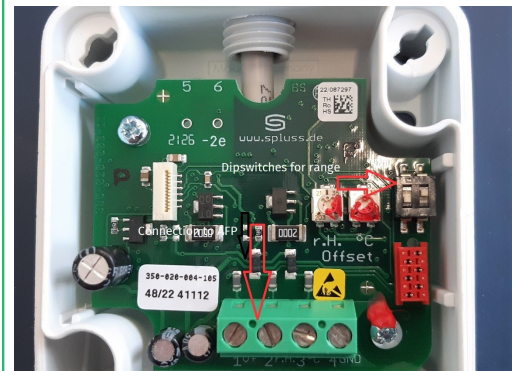
Electronic board, dipswitches for range on the right side
