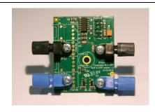
A single and a double unit have both only one power supply and only one optical fibre connection. Internally the two boards are connected, in the optical chain both are identified with their own physical address. On the outside of the housing you will see 2 serial numbers, for instance AFPD02 sr. nr. 5104, AFPD63 sr. nr. 5301
